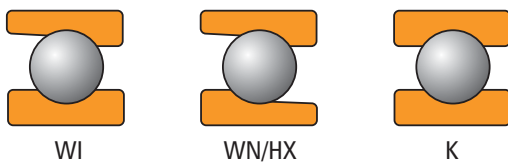
Fig. 21. Angular contact spindle bearing types.
