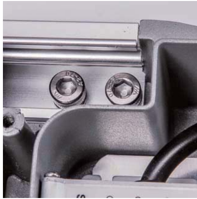
Utilize two M8 x 16 fortified stainless steel screws to fix the luminaire part to electrical part in both side
