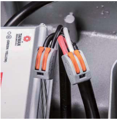
Utilize Germany WAGO connectors for output connections, safety, convenient and fast
